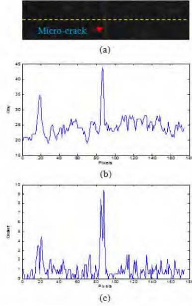
**Figure 3.** (a) The horizontal line is drawn across an area containing micro-crack pixels in Figure 2(a), (b) gray level profile of (a) and (c) gradient of (b).
