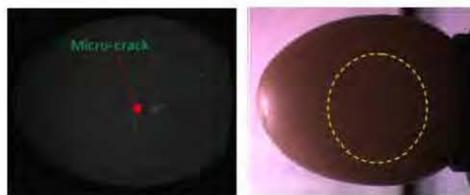
Figure 2. Example of an eggshell image with micro-crack captured using (a) candling light, (b) normal frontlighting. The dotted circle in (b) marks the area in which the micro-crack pixels are located.
